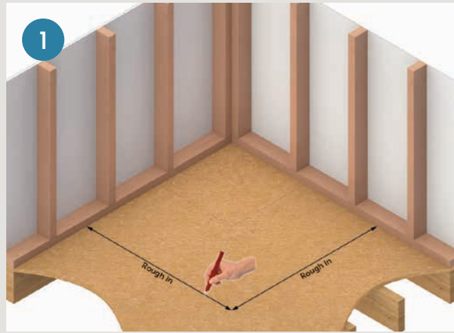
1 Mark outline of base on timber floor.
