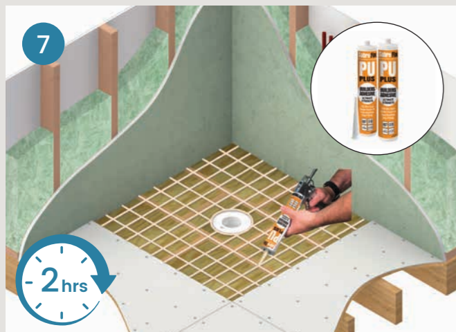
7 Fix Tile & Slate to floor outside shower pan area. Apply Polyurethane adhesive - 2 hour cure time. (Adhesive Kit included)
