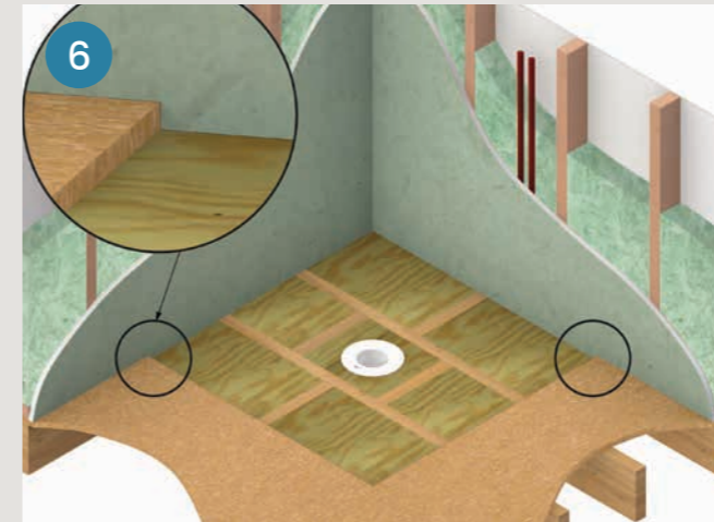
6 Install Gib/Villa board walls ensuring it follows rebate in base profile.
