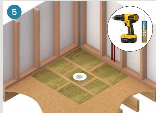
5 Infill between joists with marine ply or compressed sheet. Glue & screw into position.
