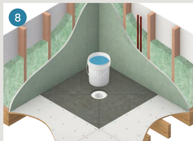
8 Fit wafer ® base and weight down with adhesive pail filled with water.
