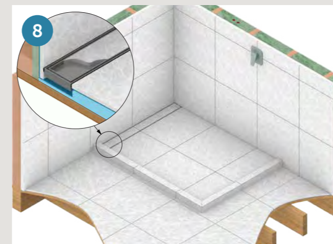
8 Fit Oben Elusion channel drain, tile insert inner pan and silicone into position.
