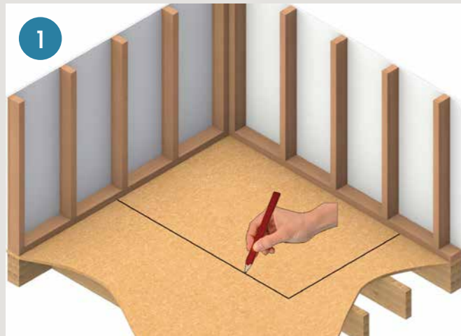
1 Mark outline of base on timber floor.
