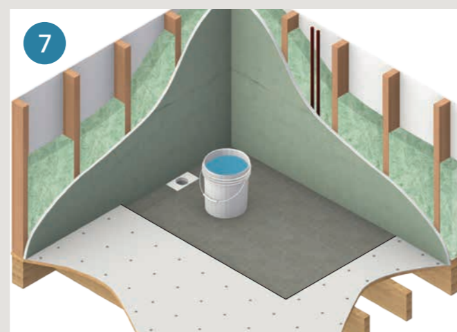
7 Install Elusion® base and weigh down with adhesive pail filled with water.
